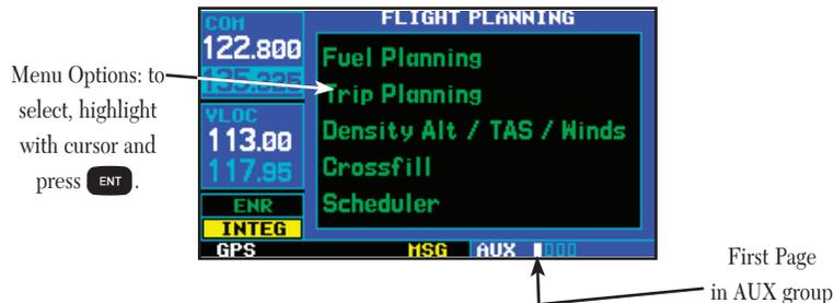
The *flight planning page* provides access (via “menu options”) to E6B functions for fuel planning, trip planning, density altitude/true airspeed/winds aloft calculations and a “Crossfill” function to transfer flight plans/user waypoints to a second GNS 430. When a menu option is selected, the corresponding page will appear providing additional information and features.
