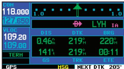
If you are in a missed approach situation, and would like to return the CDI to the 1 nm scale, activate the missed approach sequence by pressing the **OBS** key, as described on page 72. The CDI scale will also be 1.0 nm (terminal mode) within 30 nm of the departure airport.
