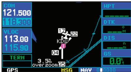
Press and hold the
