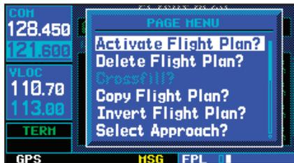
Select “Activate Flight Plan?” from the page menu to begin using the new flight plan.
