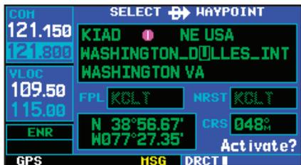
To select the direct-to destination by facility name (shown above) or city location (shown below), highlight the second or third line on the direct-to waypoint page. Use the small (⌂) and large (⌂) right knobs to enter the facility name or city. The identifier(s) for any matching entries will appear on the top line of the page.
