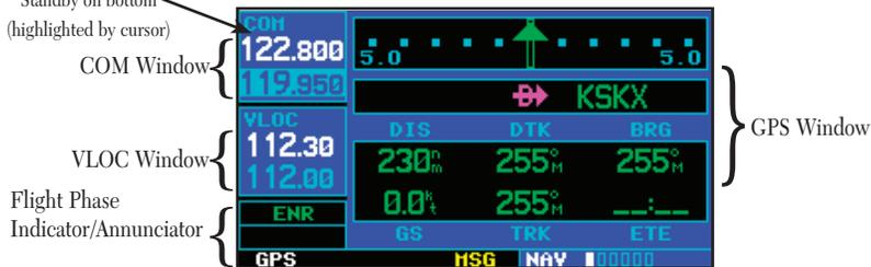
Pushing the small left knob (**[←]**) activates the tuning cursor in the desired frequency window. To select the active frequency, you must first enter the frequency in the standby field, and use the **[C]** (or **[V]**) key to move it to the active field.
