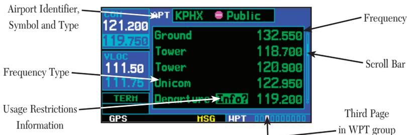
The *airport frequency page* displays radio frequencies and frequency types for the selected airport, as well as sector and altitude restrictions (where applicable). If the selected airport has a localizer-based approach, the localizer frequency(s) is also listed on the *airport frequency page*. The *airport frequency page* may be used to quickly select and tune a COM or VLOC frequency.
