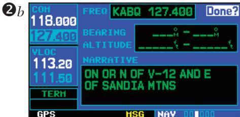
2a. Rotate the large right knob (⊖) to move the cursor through the list of frequencies. If there are more frequencies in the list that can be displayed on the screen, a scroll bar along the right-hand side of the screen will indicate which part of the list is currently being displayed.
