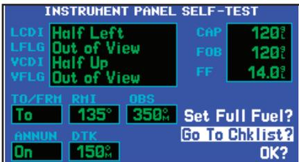
Select “Go To Chklist?” to display the checklist page and any available checklists. The GNS 430 can hold up to nine checklists with up to 30 entries in each checklist.
