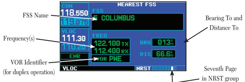
To quickly tune an FSS's frequency from the nearest flight service station page:
